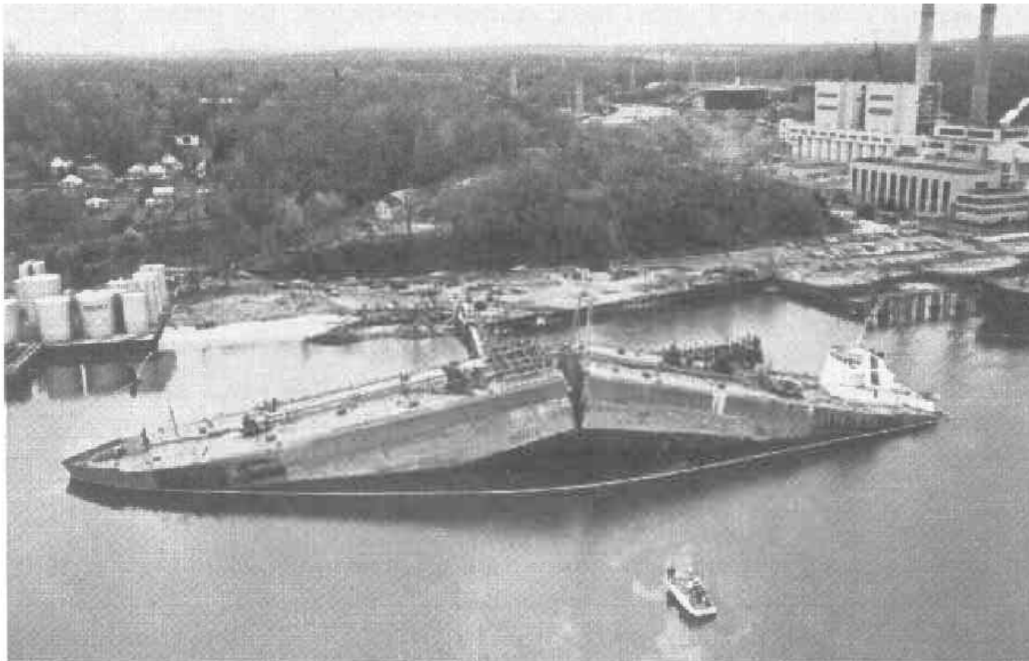
An oil barge that fractured in a brittle manner by crack propagation around its girth. (Photograph by Neal Boenzi. Reprinted with permission from The New York Times .)
